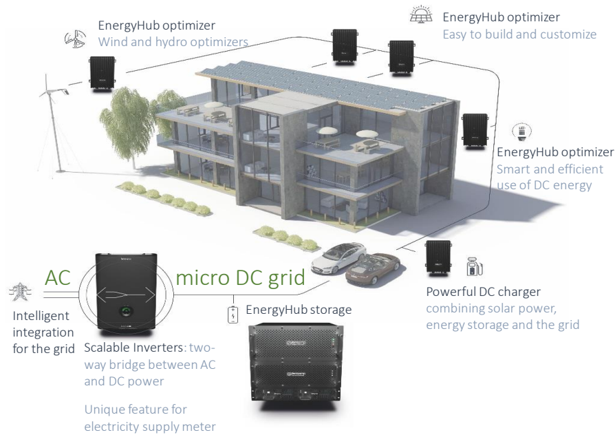
Fig. 3: Schematics of the Energy Hub micro DC grid from project partner - Ferroamp Elektronik AB
